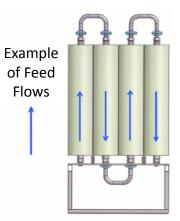
NOTE: The feed flow can be from either end of the ST+ Module BUT the Membrane Element must be installed to suit the flow direction.
