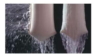
These photos clearly demonstrate the dramatic advantage of the weld liquid filter bag over coventional sewn seam bags. Conventional sewn seams contain needle holes that measure up to 1200 micron.
