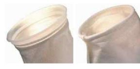
Filter bags come standard with the polypropylene collar (far left), which creates a hermetic seal within the vessel housing, preventing liquid bypass. Many other ring options are available, such as a 304 stainless steel ring (near left).
